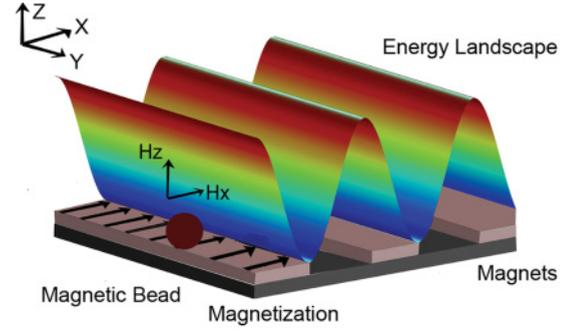
FIG. 1. (Color online) Schematic of the potential energy landscape of the bead exposed to a periodic array of micromagnets (approximated as a 1D array of infinitely long bar magnets) and external time-varying fields applied along the  $x$  and  $z$  directions. The bead is shown as a circle. The magnetization direction of the micromagnets is along the short axis.
