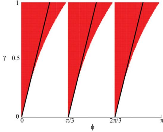
FIG. 6. (Color online) A separation window is presented to compare the direction of motion of a bead with and without static forcing terms. The red (shaded) regions indicate the phase and forcing conditions in which a bead having static terms moves in the opposite direction of one that does not. The white (unshaded) regions represent the conditions in which both beads move in the same direction. The black (solid) line is the analytically calculated separation boundary derived from Eq. (15).
