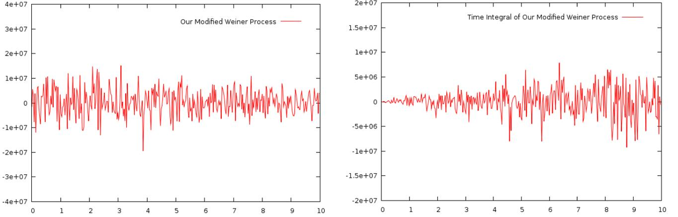
Figure 2. Plots of our modified version of the Weiner Process,  $X_t = \sigma W_t$ , where  $W_t \sim N\left(0, \xi_0 e^{-\frac{\ln(2)}{\Delta t} t}\right)$ . The left hand side depicts the Weiner Process incorporated into our energy consumption differential equation, while the right hand side plot shows its time integral, approximated using a Riemann Sum.
